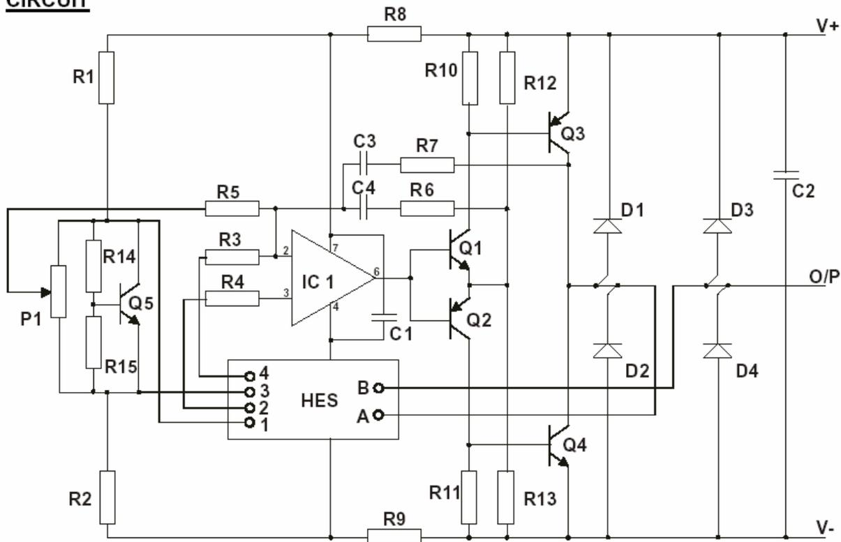
The circuit shown above and the component values given below are similar to those used in the corresponding units in the TELCON HTP/HT range.
